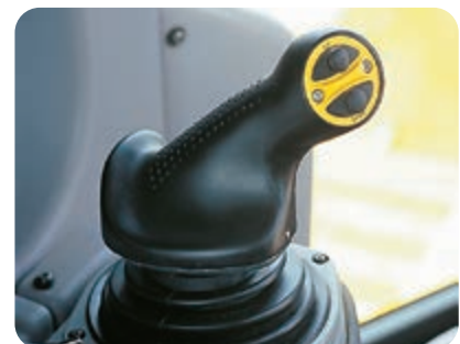
PCCS-Bedienhebel (Palm Command Control System)
