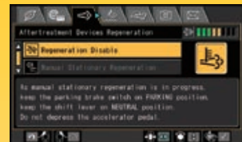
Aftertreatment device regeneration screen for the KDPF
