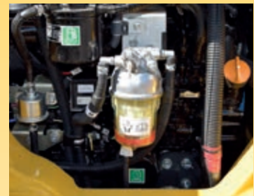
Large fuel filter and fuel pre-filter with water separator protect the engine
