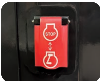
Secondary engine shutdown switch
