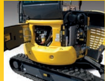
Rear bonnets for quick engine checks, simple inspections, cleaning of the radiators and easy access to the battery
