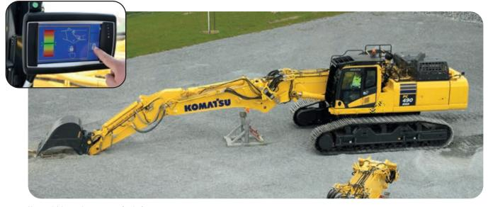
K100 quick boom change system (option) Includes Komatsu hands free boom connections, with advanced human machine interface safety system. Low profile equipment storage stands included.
