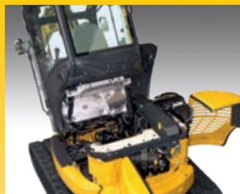
The cab easily tilts back for major maintenance tasks
