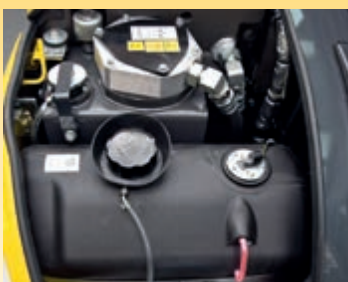
Convenient and save fuel and oil refilling under the front bonnet
