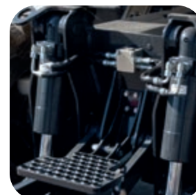
Blade/stabiliser cylinders with integrated check valve (standard)
