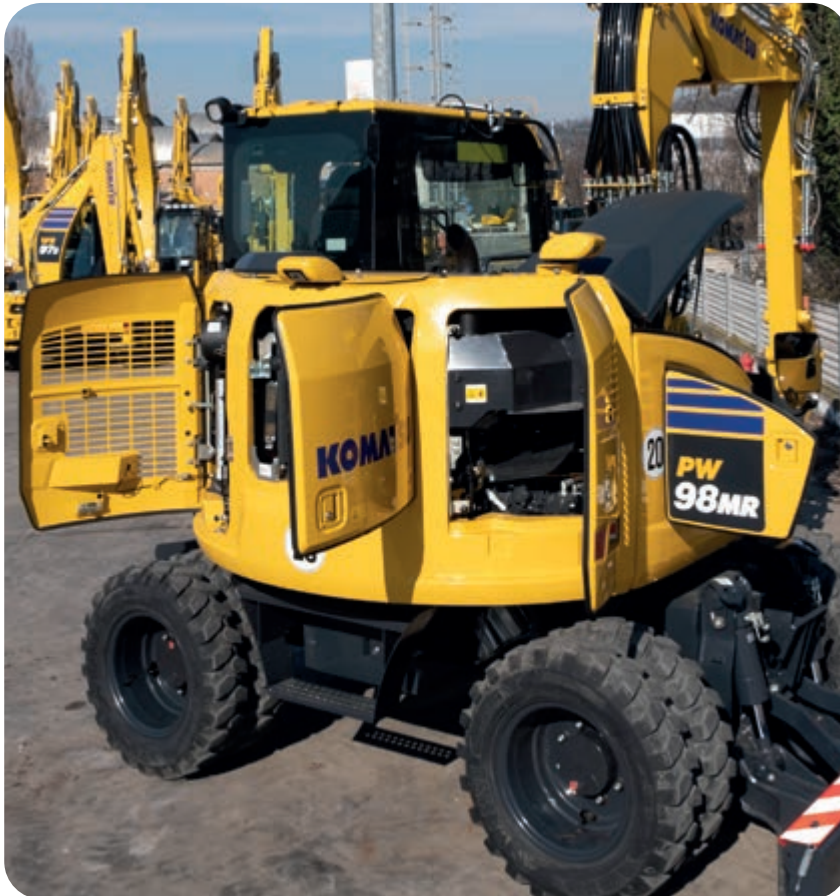
All major maintenance points can be easily reached from ground level
