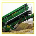
Linkage System Hydraulic Screenbox linkage system, allows greater accessibility for screen change and enables optimum screen coverage at varying screenbox angles.
