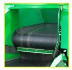
Conveyor 48" (1200mm) feed conveyor enables high capacity screening.
