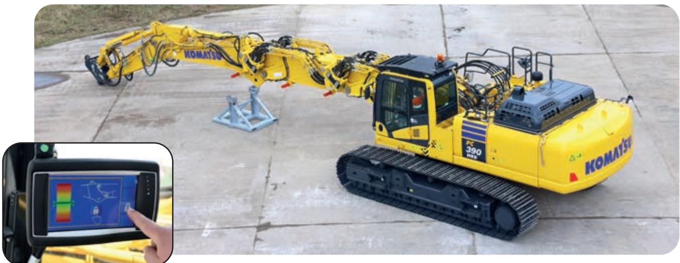
K100 quick boom change system (option) Includes Komatsu hands free boom connections, with advanced human machine interface safety system. Low profile equipment storage stands included.
